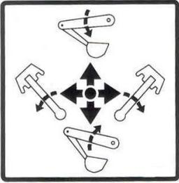
Push the left hand outer control lever, boom moves down, and pull back the lever, boom moves up. Also, pushing the lever fully forward into the detent position, allows the boom to float. In the float position, the boom can drift up or down without pressure.
