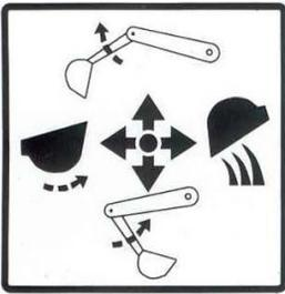
Push the right hand outer control lever, arm(dipper stick) moves away from operator, and pull back the lever, arm(dipper stick) moves toward the operator.
