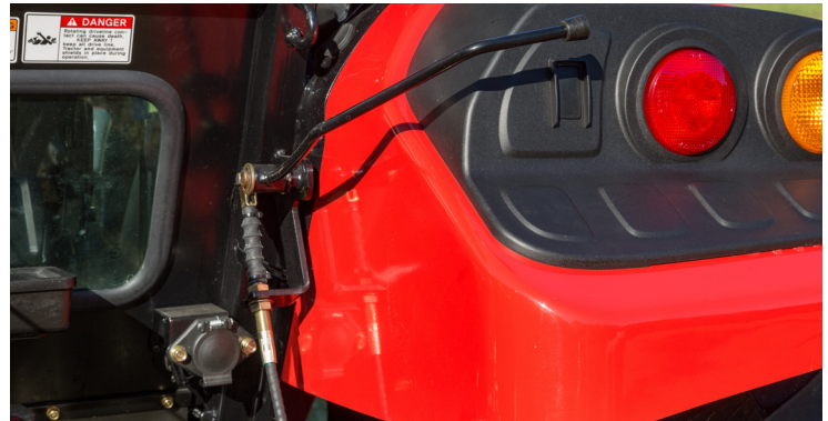
3-pt Hitch Arm Control from Rear of Tractor
